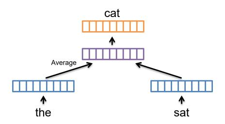
$$v_{\bar{w}_t} = \frac{1}{2c} \sum_{j=-c \& \& j \neq 0}^{c} v_{w_{t+j}}$$
